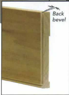
2 A flip and a plunge. The baseboard then is flipped upside down on edge, and the saw is plunged down the straight part of the profile at a slight back bevel.
